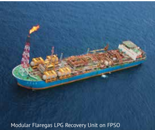
Modular Flaregas LPG Recovery Unit on FPSO
