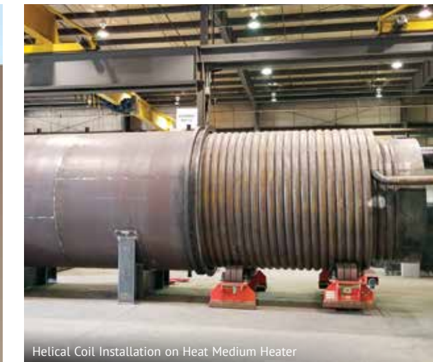
Helical Coil Installation on Heat Medium Heater
