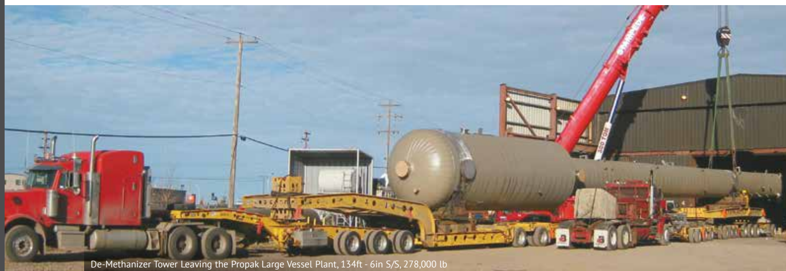
De-Methanizer Tower Leaving the Propak Large Vessel Plant, 134ft - 6in S/S, 278,000 lb
