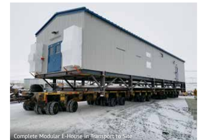
Complete Modular E-House in Transport to Site
